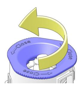
9. Place the grinder house top assembly, and turn it in the direction of the arrow to lock.
