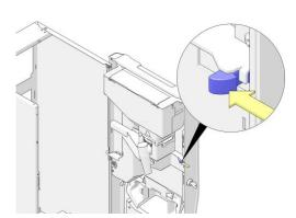
2. Press the **locking lever** to unlock the canister door.
