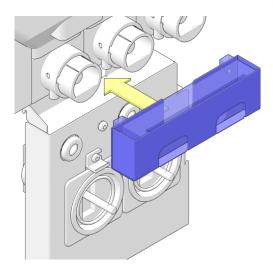
14. Install the bayonet catches and turn clockwise (approx. 10°).
