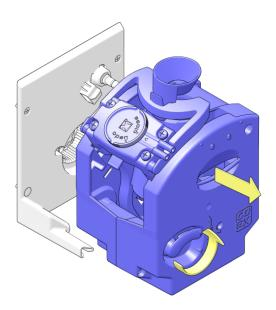
3. Push the fixation handle upwards and, while keeping the handle in the upward position, pull and lift the brewer in the direction of the arrow out of the coffee machine.
