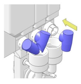
18. Install the canister outlets on the canisters and make sure the locations and positions are correct.
