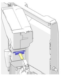
12. Push the canister locking slider back to lock the bean canister on the grinder base.
