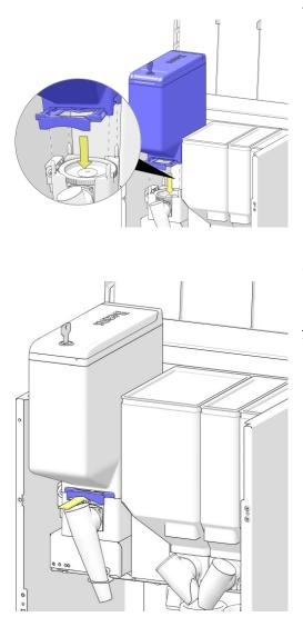
10. Place the bean canister back into the coffee machine on the four position ridges of the grinder base.
