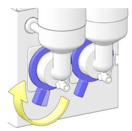
17. Turn the bayonet catches clockwise to lock the mixer houses.
