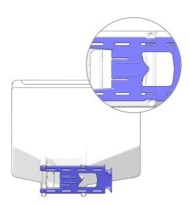
4. Locate the canister locking slider in between the grinder and the bean canister.
