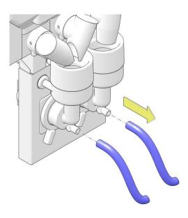
2. Remove the canister outlets and remember the correct position and location of each outlet.
