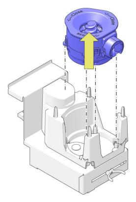
5. To clean the D-grinder, lift and remove the grinder from the base.
