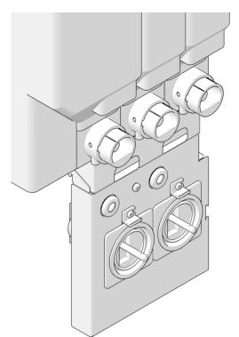
12. Insert the mixer exhaust filter in the filter drawer.
