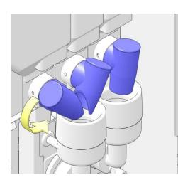
9. Turn the outlets of the canister downwards.
