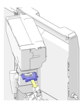
5. Pull the canister locking slider in the direction of the arrow. The bean canister will be closed and unlocked from the grinder base.
