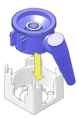
4. Place the grinder back into the grinder base and continue with step 12.
