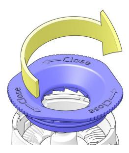
7. Loosen the bayonet locked grinder house top in the direction of the arrow and remove it from the grinder.
