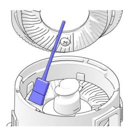
8. Clean both grinder discs and the inside of the grinder house.
