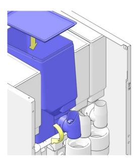
8. Place the lid back on the canister and position the canister back into the machine.
