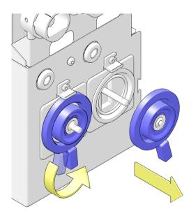
6. Turn the bayonet catches counterclockwise (approx. 10°) again to release and pull them in the direction of the arrow away from the machine.
