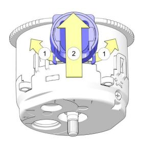
6. Pull out the clips of the grinder outlet (1), slide the outlet from the grinder house (2) and remove it from the grinder.
